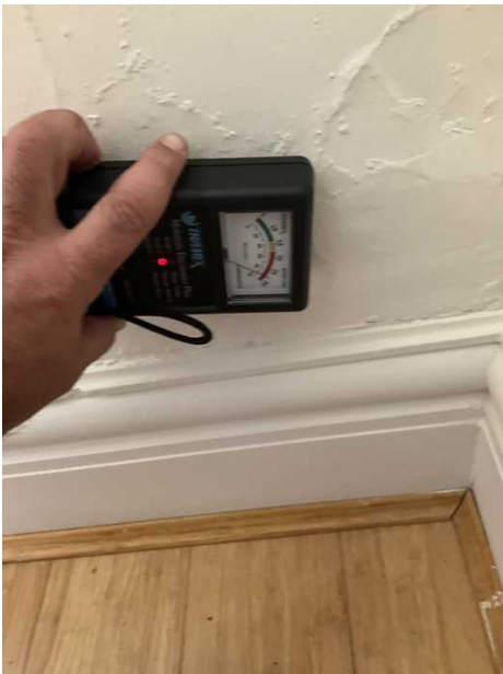
Example of high moisture reading to main bathroom walls,
