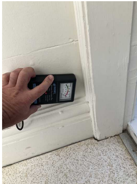
Example of high moisture reading to laundry/ bathroom shower walls.
