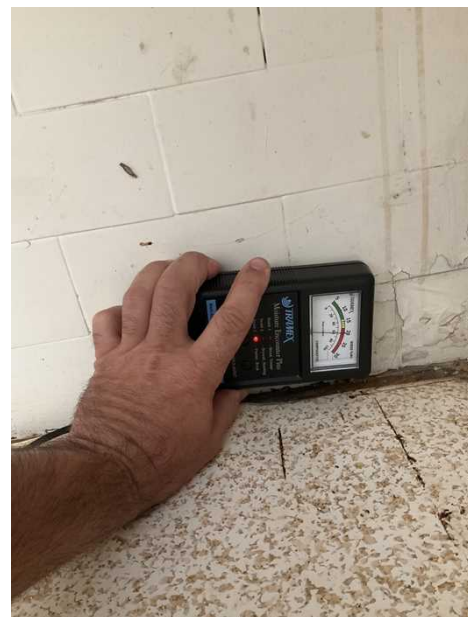
High moisture readings to areas. Recommend engaging a builder for invasive inspection to determine moisture source., + High moisture readings to Laundry/bathroom shower walls.
